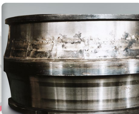
Bearing damage caused by lubrication starvation
